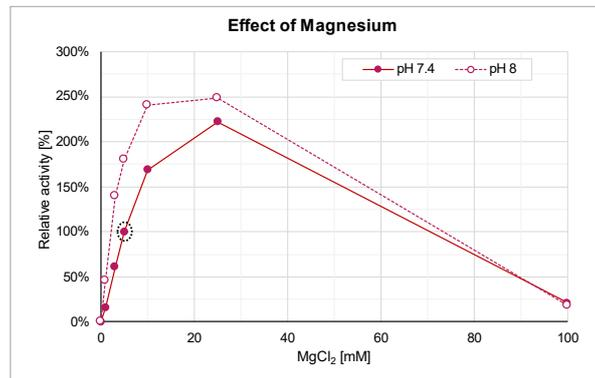
**Fig. 3** Effect of low to high MgCl<sub>2</sub> concentrations on enzyme activity of DENARASE High Salt at 250 mM NaCl. The volumetric activities at pH 7.4 and pH 8 were measured in U/ml and normalized to activity at 5 mM MgCl<sub>2</sub> and pH 7.4 (indicated by dotted circle).
