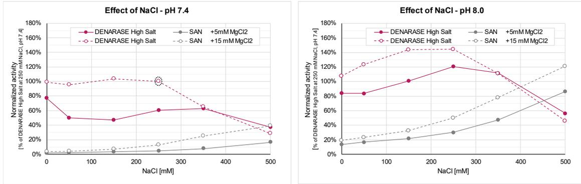
**Fig. 2** The effect of increasing NaCl concentrations on the enzyme activity of DENARASE High Salt and Salt Active Nuclease High Quality (SAN, ArcticZymes). The volumetric activities at pH 7.4 (left) and pH 8 (right) were measured in U/ml. After normalization to the activities as given on the CoAs of the respective enzyme batches, enzyme activities were normalized to DENARASE High Salt activity at 250 mM NaCl, 15 mM MgCl<sub>2</sub> and pH 7.4 (indicated by dotted circle).
