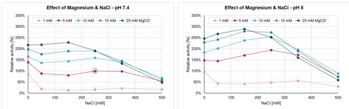
**Fig. 4** Effect of low to intermediate MgCl<sub>2</sub> levels in combination with 0-500 mM NaCl on enzyme activity of DENARASE High Salt. The volumetric activities at pH 7.4 (left) and pH 8 (right) were measured in U/ml and normalized to activity at 250 mM NaCl, 5 mM MgCl<sub>2</sub> and pH 7.4 (indicated by dotted circle).
