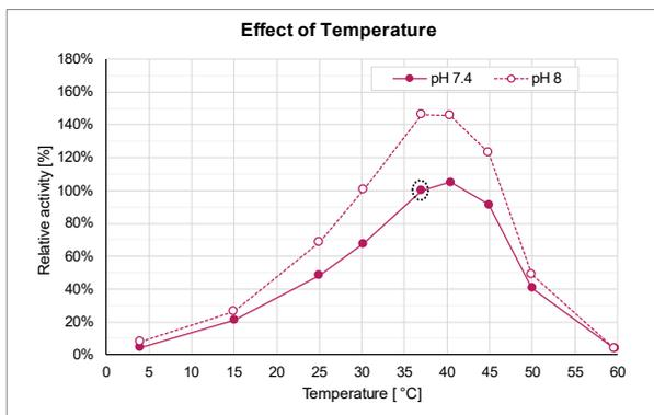
**Fig. 6** Effect of temperature on DENARASE High Salt activity. Enzyme activity at different temperatures at pH 7.4 and 8.0 were normalized to activity at 37 °C, 5 mM MgCl<sub>2</sub> and pH 7.4 (indicated by dotted circle).
