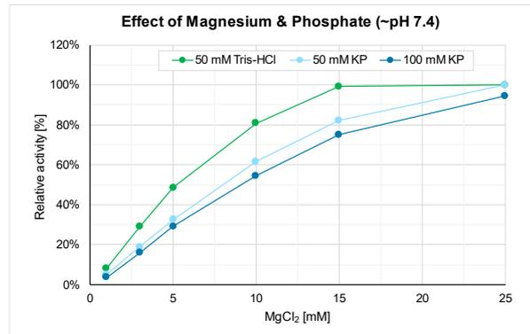
**Fig. 5** Effect of MgCl<sub>2</sub> on DENARASE High Salt activity in Tris-HCl and potassium phosphate (KP) buffers. Volumetric activities at 250 mM NaCl were measured in U/ml and normalized to maximal enzyme activities.
