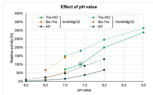
**Fig. 7** Effect of pH on DENARASE High Salt activity. Enzyme activities in Tris-HCl, Bis-Tris and potassium phosphate (KP) buffer at different pH levels in the presence of 5 mM and 15 mM MgCl<sub>2</sub> were normalized to DENARASE High Salt activity at 5 mM MgCl<sub>2</sub> and pH 7.4 (indicated by dotted circle).
